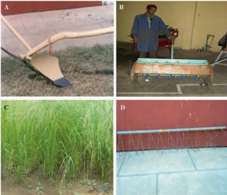
Fig 1. Implements developed or tested for various cultural practices involving tef. A) Erf and Mofer attached moldboard plow; B) Seed drill; C) Performance of tef plants sown by the seed drill indicated in B; D) Part of the modified pickup reel developed or tested for tef harvesting.
